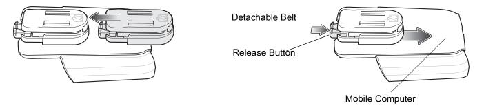
Figure 67 Attaching the Rigid Holster
